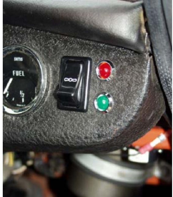
LED mounted in the crackle finish dashboard alongside a cooling fan override switch and green LED
